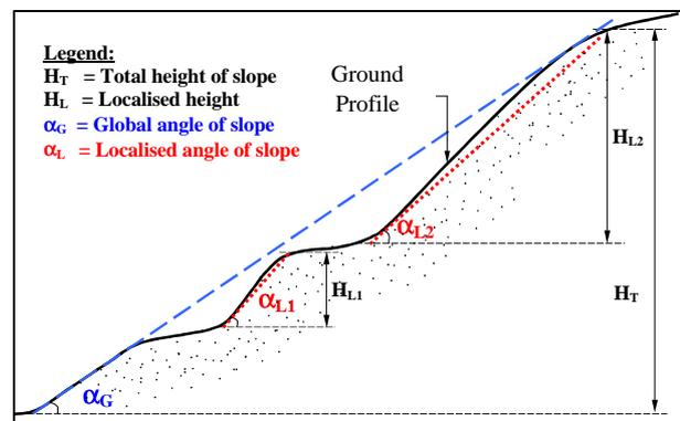
Figure 1 : Geometries of Slope (after IEM, 2000)
