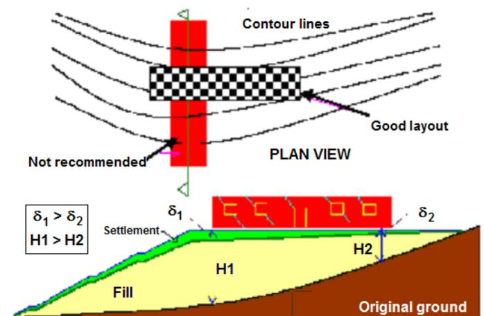
Figure 7.4. Different layout of building on filled ground.
