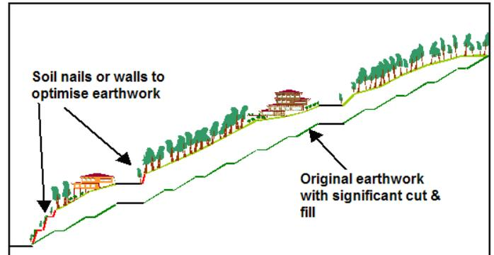
Figure 7.2. Method to optimise earthworks.
