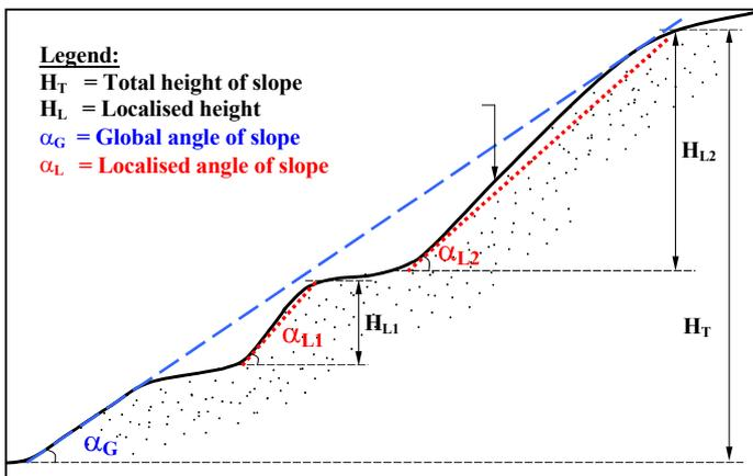
Figure 7.1. Geometries of slope (after IEM 2000).
