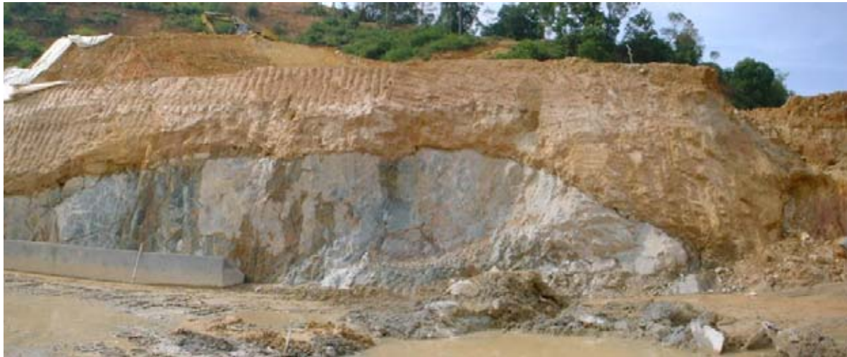
Figure 10: Inconsistent Weathering Profile (After Liew S.S. 2005)
