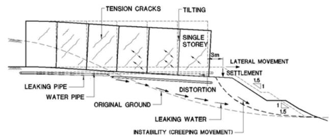
**Figure 7 Building Distortion due to Differential Fill Settlement**
