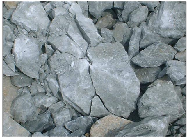
**Plate 4 Breakage of Rock Fragment under Heavy Compaction**
