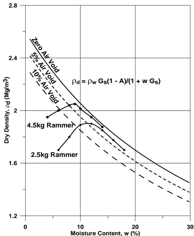
Figure 1 Dry Density-Moisture Content Relationship with Compaction Curves
