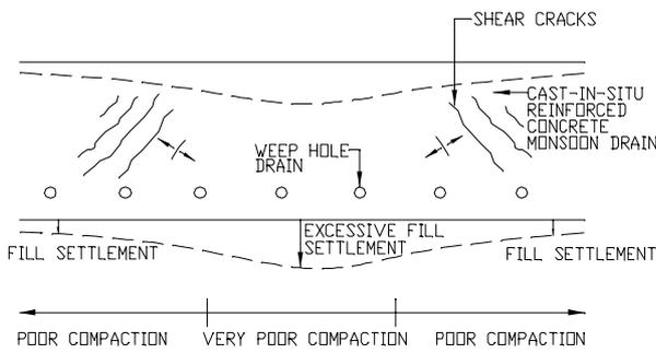
**Figure 6 Shear Cracks on Monsoon Drain**
