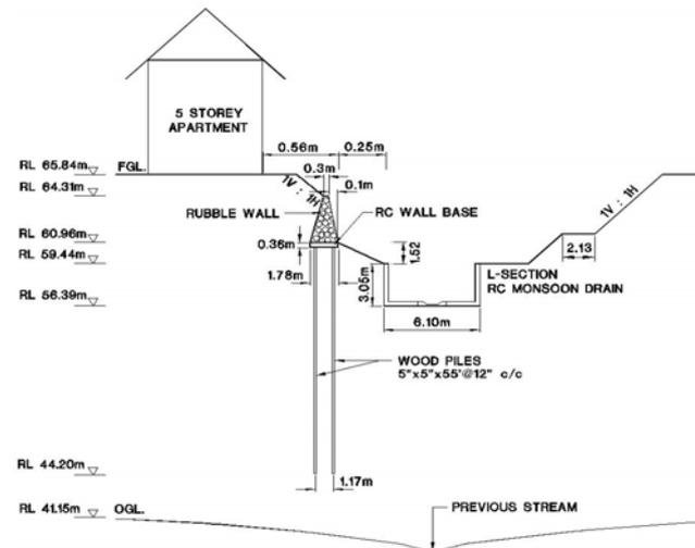
**Figure 5 Cross Section of the Rubble Wall and Monsoon Drain**
