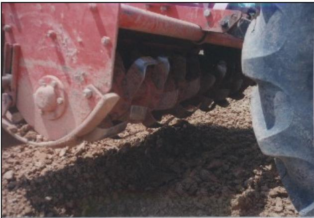
**Plate 3 Scarifier Mounted to Back-Pusher**
