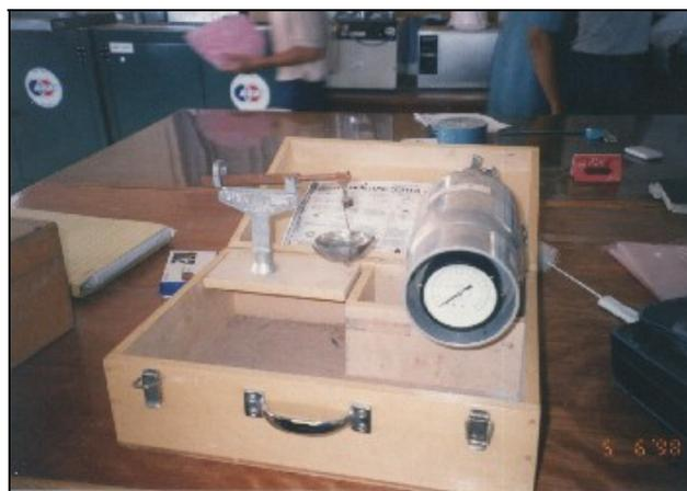
**Plate 1 Speedy Tester for Quick Determination of Moisture Content at Site**
