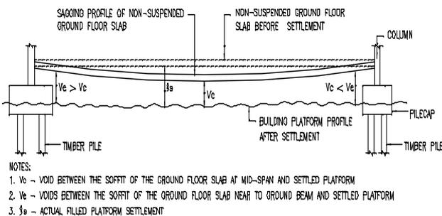
Figure 3 Sagging Ground Floor Slab
