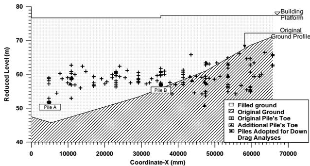
**Figure 4 Pile Penetration Records**
