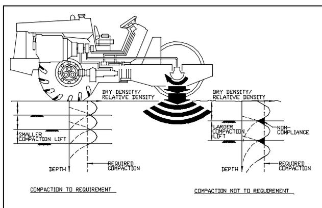
**Figure 2 Control of Loose Lift Thickness**
