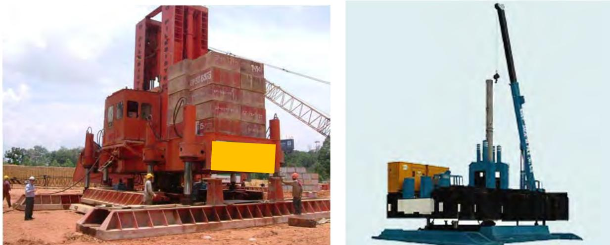
Figure 1. Typical high capacity jack-in pile machine in Malaysia.
