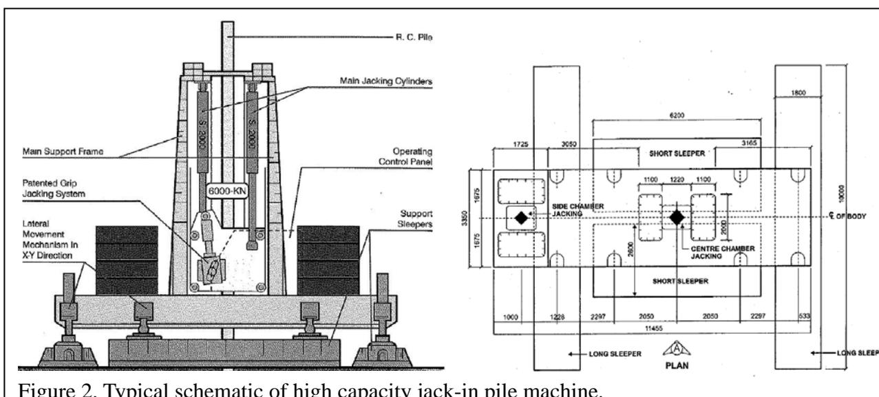
Figure 2. Typical schematic of high capacity jack-in pile machine.
