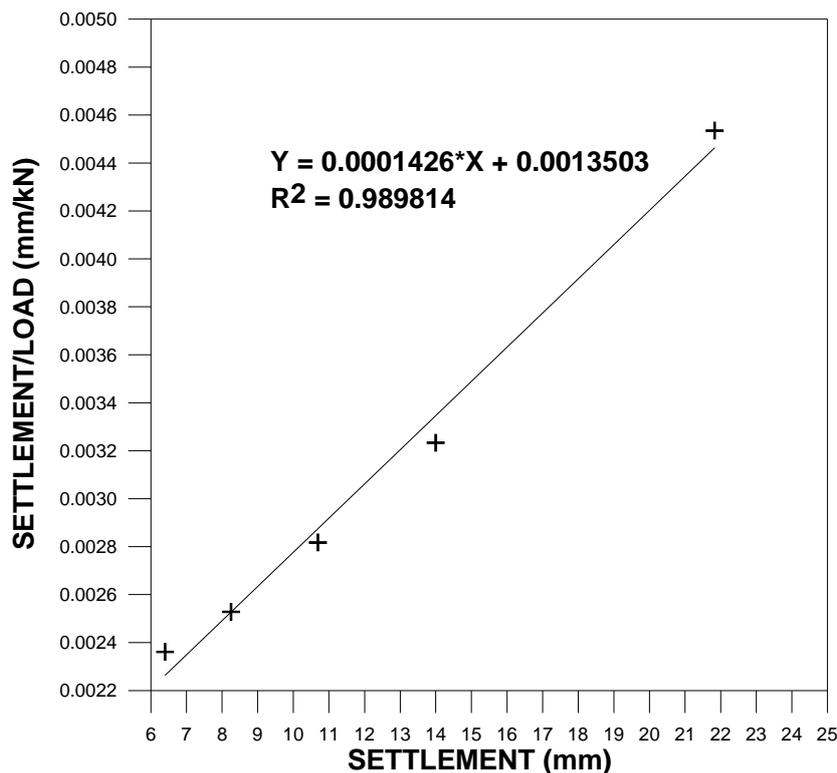
Figure 13. Chin’s plot for  $\phi$ 500mm spun pile (Site D).
