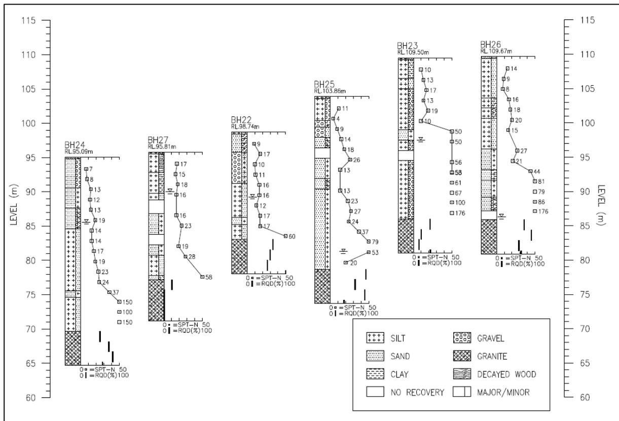
Figure 6. Borehole profiles at Site B.
