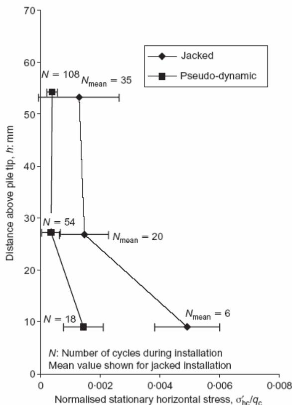
Figure 3. Influence of loading cycles during installation on stationary horizontal stress (White & Lehane, 2004).
