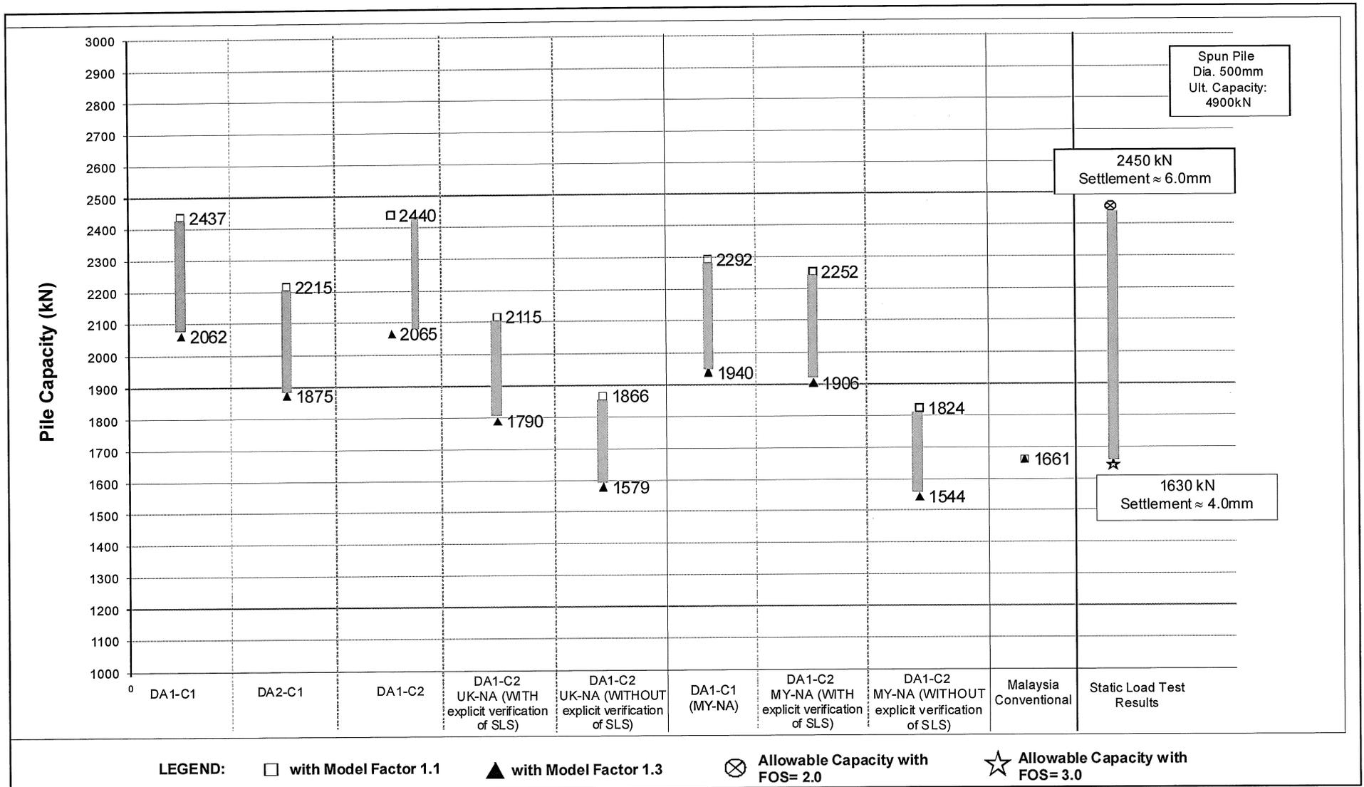
Figure 14. Allowable pile capacity of Jack-in Pile calculated using various methodologies compared with the Malaysian conventional design method and static pile load test results ( $\phi$ 500mm Spun Pile – Site D).
